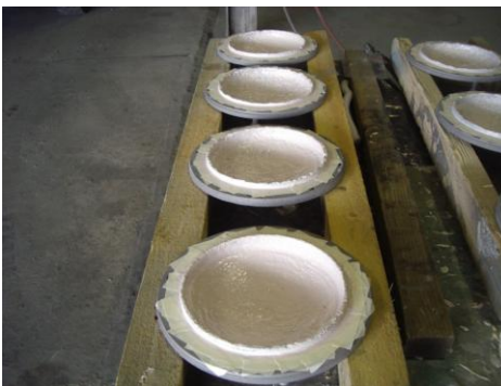
Covers after first coat with RB 332
