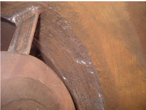
Pitting and erosion in the wear spacer ring/housing
