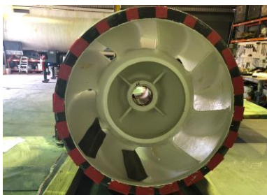
Reinforcing diffuser leading edges
