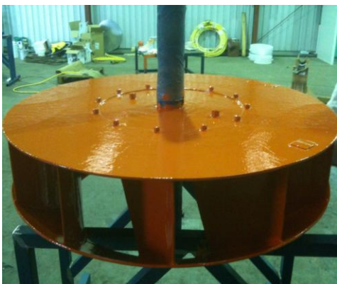
Completed coated and balanced fan using RS 500P & RU 500
