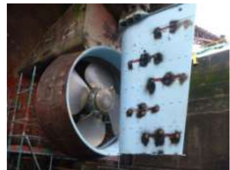
After 18 months in service: Coating still in perfect condition
