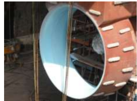
Chem-glide™ RA 500CG applied to Kort Nozzle
