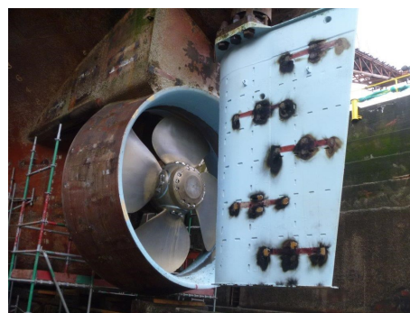
After 18 months in service: Coating still in perfect condition
