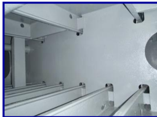
Full surface coated with RS 500P, including all sharp edges, corners and weld areas
