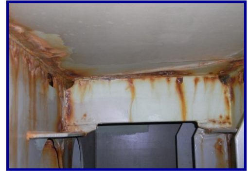
Double-bottom tanktop after 7 years in-service
