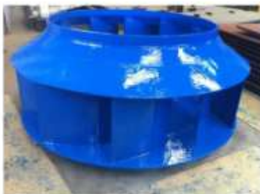
View of impeller completion
